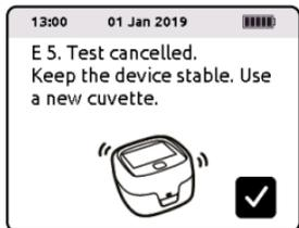
The measurement can not be made because the device is not level. The test has been cancelled.
