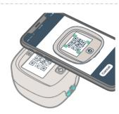
**14.** Press the **D** button to reveal the QR code. If you are using the Luma app, scan the QR code to upload and track your results.
